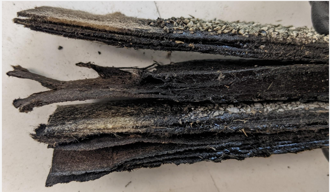
Figure 16: Solvated samples - from bottom to top - Firehall, Alfred Jenkins, Police Station, Municipal Services Centre.
